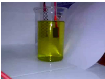
Fig. 4. Sol-Gel interface formed at cathode during chitosan electrodeposition.
